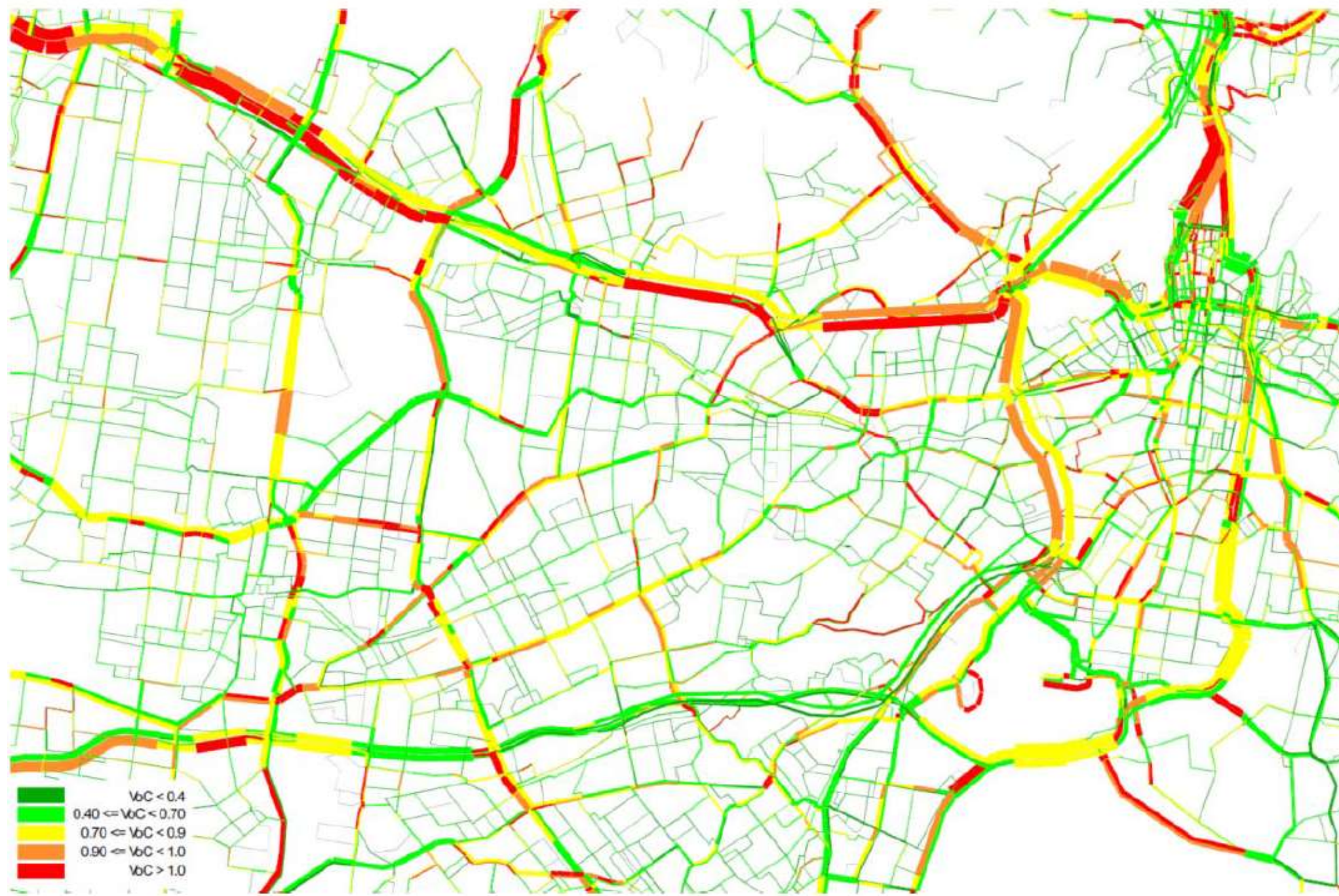
Figure 7-1 Link volume to capacity ratio on the network following WestConnex and Western Harbour Tunnel, 2031 morning peak
